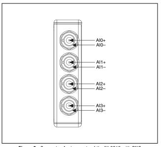
Figure 3. Connector Assignments of the NI 9215 with BNC
